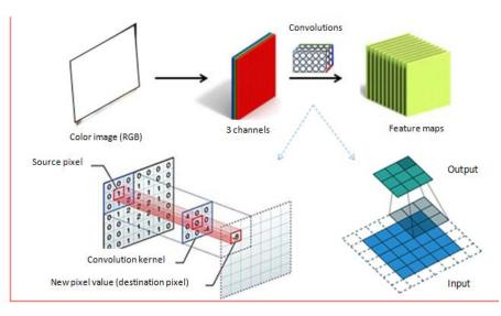
Figure 1: Operation of convolutional neural networks.
