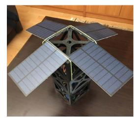
Figure 7: Nanosatellite prototype.
